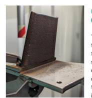
Layer-by-layer structure of the prong on the robotic arm of the Additive Mobile Factory®
