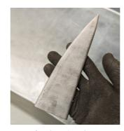
Prong for the mine clearance machine, printed using the cladding method
