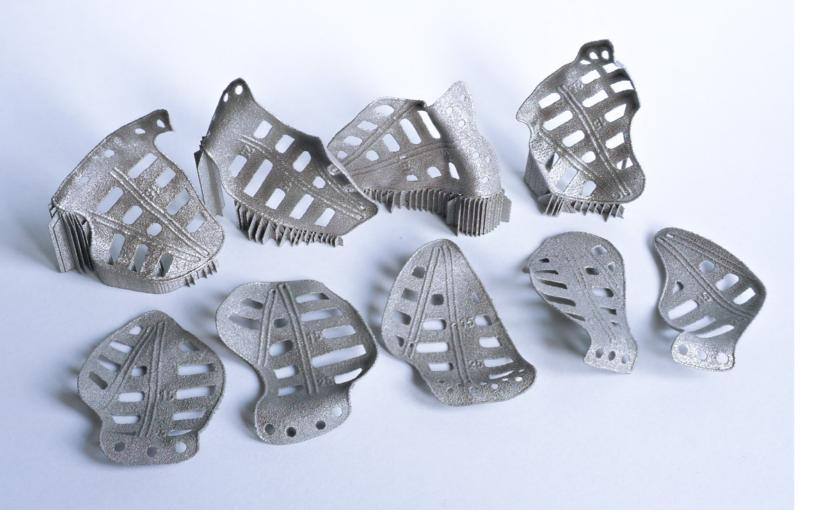
A continuous process chain for manufacturing patient-specific implants was automated for the first time
